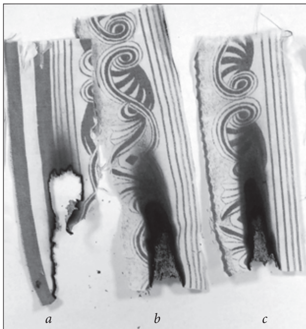
Fig. 4. Fabric samples after vertical flame test: a — PhA treated; b — PhA + allantoin treated; c — PhA + allantoin + aluminum sulfate treated
