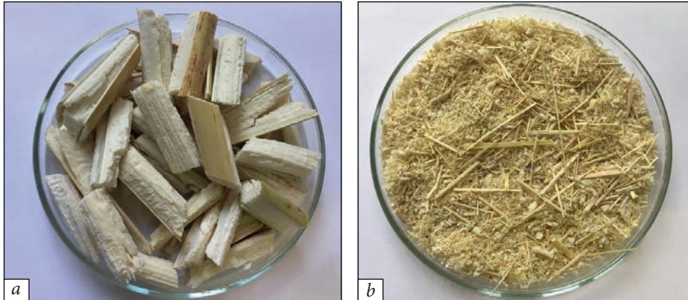
Fig. 2. Sweet sorghum bagasse: a — chopped into 2.5–3 cm long pieces approximately; b — finely ground
