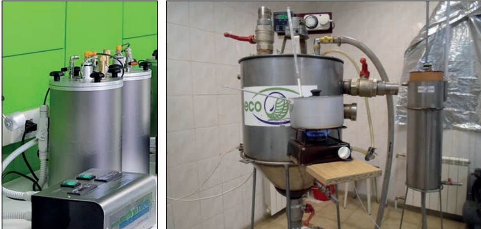
Fig. 3. Methane Tube setup for rapid determination of biogas yield from various substrates. The installation includes a biogas reactor with a working volume of 30 dm 3 and is located at the NUBiP
